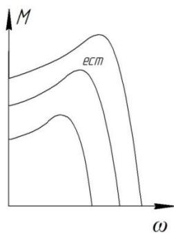
$$\begin{aligned}\frac{U}{f} &= \text{const} \\ + f \\ \frac{U}{f^2} &= \text{const} \\ \frac{U}{\sqrt{f}} &= \text{const} \\ f = \text{varia} \quad U &= \text{const}\end{aligned}$$
