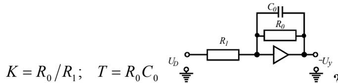
$$K = R_0 / R_1; \quad T = R_0 C_0$$
