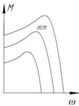
$$\begin{aligned}\frac{U}{f} &= \text{const} \\ + \frac{U}{f^2} &= \text{const} \\ \frac{U}{\sqrt{f}} &= \text{const} \\ f = \text{varia} \quad U &= \text{const}\end{aligned}$$
