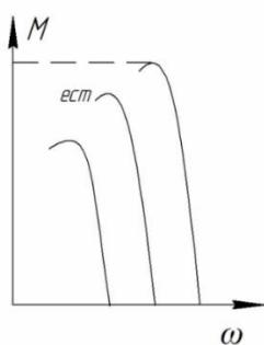
$$\frac{U}{f} = \text{const} \\ +f \\ \frac{U}{f^2} = \text{const} \\ \frac{U}{\sqrt{f}} = \text{const} \\ f = \text{varia } U = \text{const}$$
