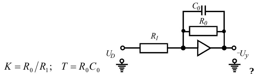
$$K = R_0 / R_1; \quad T = R_0 C_0$$
